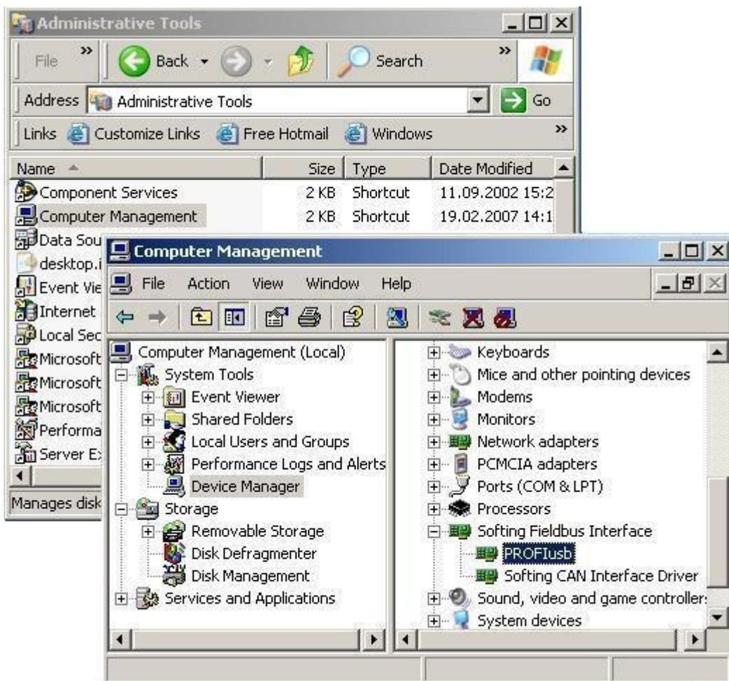
The interface is installed correctly when it is displayed in Device Manager as shown above.
